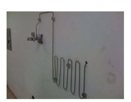
Coiled tube to stabilize the temperature of the detector gas (the gas cylinder is outside the lab)
